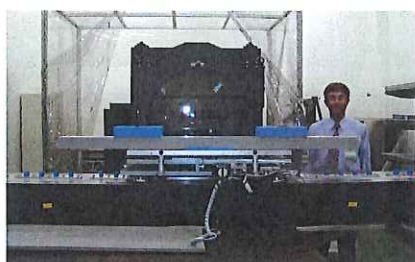
Measuring Instrument : ZYGO32 ( \phi 800 ) Interferometer
