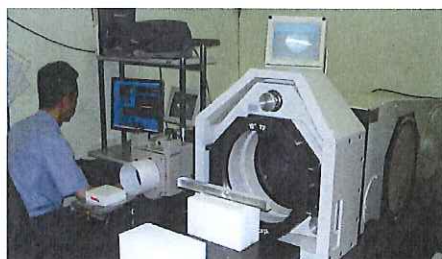
Measuring Instrument : ZYGO12" ( \phi 300 ) Interferometer
